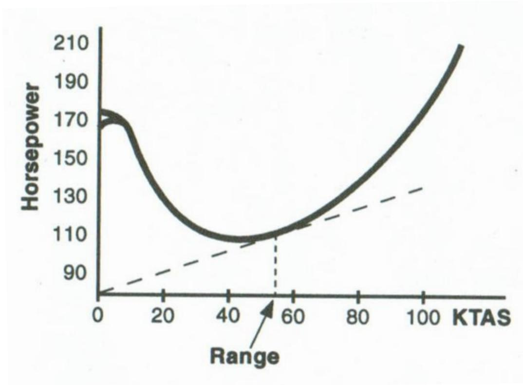
The Horsepower required Graph shows pilots the engine horsepower required to maintain level flight at a given speed. Using this Graph allows us to establish airspeeds to fly at minimum power or the speed to achieve maximum range
